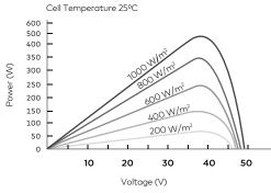
P-V Curve at Different Irradiation (530 W)
